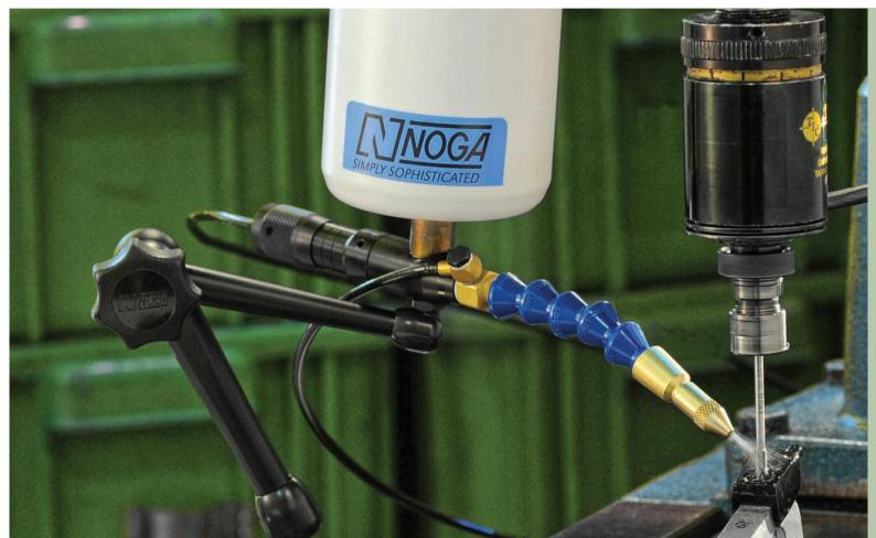
**COBRA 's** drop ejector is designed to accurately shoot small quantities of liquid to distinct targets. An air actuated piston shoots the drops through a flexible hose onto the target.
